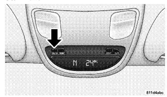
Use this button to change the display from U.S. to metric measurement units.
